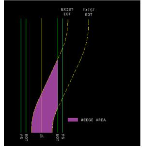
Our Corridor Modeling Templates use a special innovative point constraint to the achieved this desired effect. "Horizontal Minimum" is used to control the horizontal widening/wedging limits for the following two conditions.
