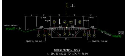
What happens in the same scenario when the existing EOT is located outside the proposed EOT? The wedging then stops at the proposed EOT and does not get carried over to the proposed paved shoulders. Below is an illustration of areas suitable for wedging.
