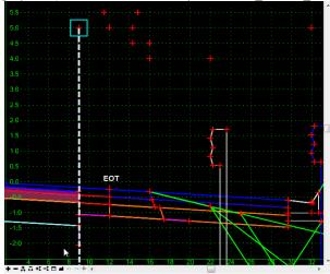
When the existing EOT is located outside the proposed EOT point, widening/wedging occurs up to the proposed EOT point (horizontal location of point "PV1\_OEOT").
